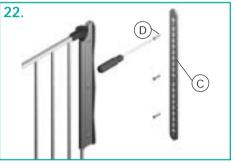
Note: Screws provided are for mounting directly into wood. If mounting into brick, drywall or other surfaces, use appropriate hardware.
